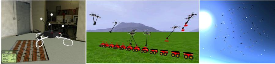
Fig. 3: Three screenshots taken from different simulations. *Left*: simulated quadrotor during the *physical fidelity* test. *Center*: stroboscopic sequence of a cooperative-aerial grasping performed by a quadrotor and a ground robot. *Right*: 70 quadrotors performing autonomous formation control on a spherical surface during the *real-time capabilities vs. number of robots* test.
